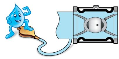
When no pressure acts on the valve, the resilient heavy duty sleeve holds the **Inbal** valve closed.
