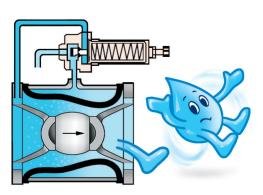
The **Inbal** Valve opens quickly as soon as the line pressure exceeds the setting. Once the pressure surge is safely dissipated, the **Inbal** Pressure Relief Valve closes tightly in readiness for the next excess of pressure.
