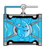
The **Inbal** Valve closes when inlet pressure is applied to the control chamber. The equilibrium in pressures and forces acting on the sleeve maintains the valve in a closed position.
