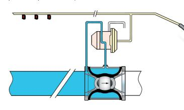
control service). The pneumatic (pilot) actuator enables an effective control to open and close the **Inbal** Valve even by very low air or gas pressure. In most applications, loss of the dry pilot line pressure will open the **Inbal** Valve, but there are applications where pneumatic pressure is provided to open the **Inbal** Valve.
