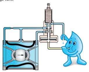
Once the release system is activated, the opening of the **Inbal** Deluge Valve is of modulating action to maintain the delivery pressure at the preset level.
