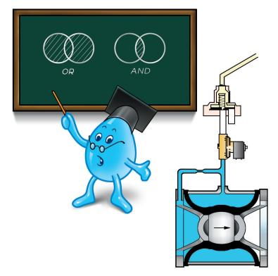
Non-interlock pneu-electric release control. The **Inbal** Valve will open either upon the operation of the electric release or a drop of pressure in the dry pilot line.
