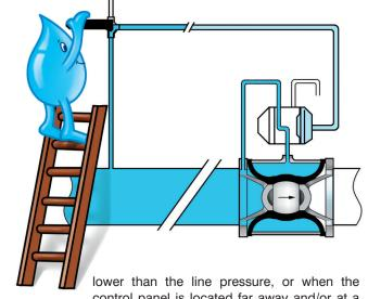
control panel is located far away and/or at a higher elevation, a hydraulic actuator (or hydraulic pilot actuator) is added to the **Inbal** Valve control.
