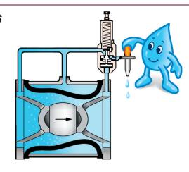
thus the incoming and outgoing flow rates to the **Inbal** Valve control chamber are equal.
